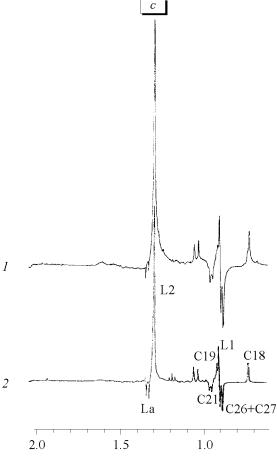
**Fig. 1.** High-field regions of spin-echo (a,c) and single-impulse PMR spectra (b) of human plasma (a) and its methanol extracts (b,c): 48-h oxidation with  $CuSO_4$  (1) and control (2). Signals: L1 and L2,  $CH_3$  and  $(CH_2)_n$  of lipoprotein lipids, respectively; Val, valine; La, lactate; Ala, alanine; N-Ac, N-acetyl terminal groups in  $\alpha_1$ -acids of glycoproteins; C18, C19, and C26+C27,  $CH_3$  groups of cholesterol.
